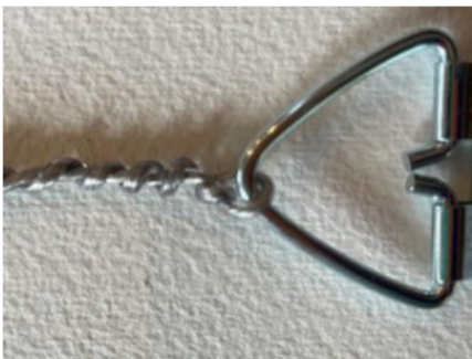
Fig. 2- Slip knot with ends wrapped.
